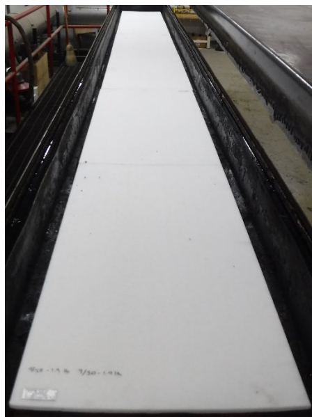
Photo No. 2 Unexposed Surface of the Test Specimen (Pre-test)
