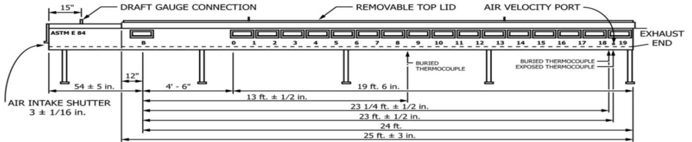
**Diagram 1.** Test Chamber side view showing critical dimensions.
